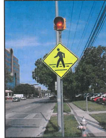
Flashing pedestrian yield sign. www.pedbikeimages.org/ (Dan Burden)
